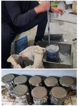
Fig.2 The molding process of concrete materials
