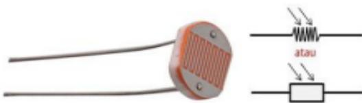
**Gambar 2.6 Light Dependent Resistor**
