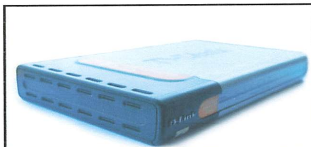
Gambar 3.3 HUB D-LINK 8 port
