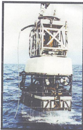
Gambar 2.2 Cable Repair Systems (Pike, 2001)
